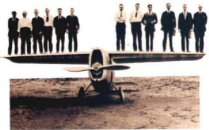
The RB Racer, made by Davton-Wright Airplane Company, was the first aircraft to have fully retractable landing gear. Dayton-Wright became an early part of General Dynamics.
