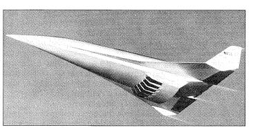
The National Aerospace Plane's supersonic combustion "ramjet" engine would eliminate the need for external rockets.
