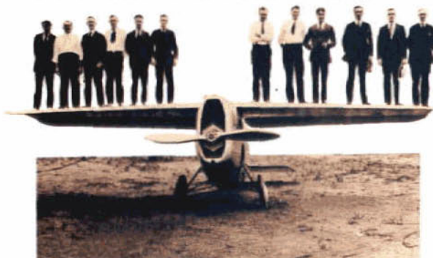
The RB Racer, made by Dayton-Wright Airplane Company, was the first aircraft to have fully retractable landing gear. Dayton-Wright became an early part of General Dynamics.
